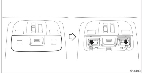
(2) Release the clips and pull out the light assembly - map to disconnect the connectors.
